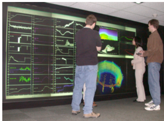
Figure 1. Tiled display walls with shared visualizations and communication are being prototyped for a collaborative fusion experimental control room.
